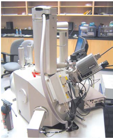
The Roentec silicon drift detector is a new and important attachment, pictured at the right of this scanning electron microscope, negating the need for liquid nitrogen to operate the MLA system.
